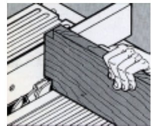
Fig. 4. Using dado to cut tenons (note use of extension fence.)
