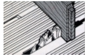
Fig. 5. Cutting the opening for drop-leaf supports 1/2 of the depth at a time.
