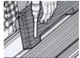
Fig. 6. Drilling screw pockets in sides. Drilled at 10-degrees with a 1/2" Forstner bit, to within 3/8" of the bottom. Use a 1/4" brad-point bit to make pilot hole for the #12 roundhead screws.
