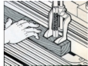
Fig. 3. Cutting mortise in leg (note hold-down).
